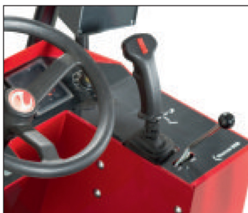
On the Norcar 765, travel direction is chosen using a switch on top of the joystick.
